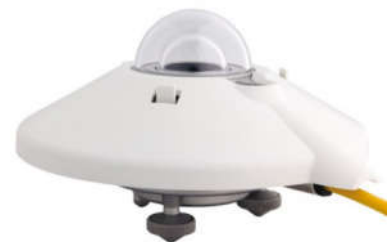
Figure 3.8 – Pyranometer. Source Own author
