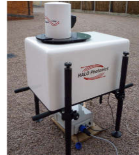
Figure 3.5 – Doppler lidar. Source: Own author
